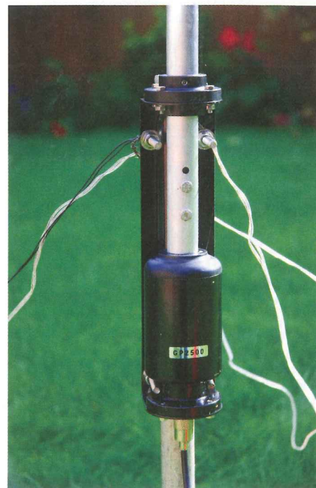
PHOTO 2: At the bottom of the antenna is a sealed matching unit with an SO239 socket for connection to the coax.
